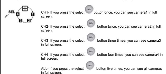
Quad screen: Images from all 4 cameras are displayed at the same time in 4 separate sections on a single screen.
